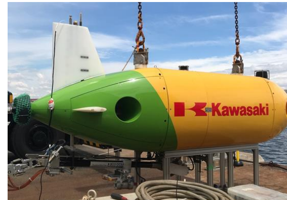
AUV equipped with All Polymer Batteries
