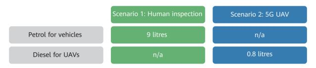
The fuel economy of UAVs is significantly better than that of petrol-powered vehicles: while a litre of petrol can sustain a vehicle for around 6km on average, a litre of aviation diesel can power a UAV for 195km, more than enough for one routine inspection. Given that UAVs also take the optimal route, the amount of fuel required for one round of inspection is very substantially reduced.
