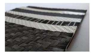
Inspired by **nature**, CompPair Technologies Ltd. brings the **healing capability** to composites. Our vision is to bring **full circularity** to the composite industry, **extending the lifetime of composites by healing matrix** and enabling a **more efficient recycling** of the fibers at the end of life. HealTech<sup>™</sup> products by CompPair are **pre-impregnated textiles** available with multiple architectures and fibre types (see page 4 for more information).
